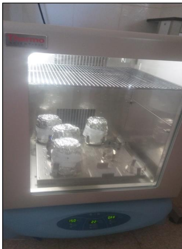
Figure 18 : Precise Shaking Incubator (Rouari, 2022).
