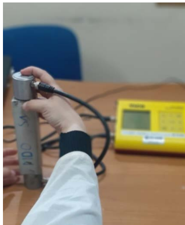
Figure II.8 : Essai Auscultation sonore
