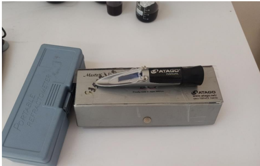
Figure 12 : Refractometer (ATAGO Master- \alpha "Alpha"). (Original, 2025)
