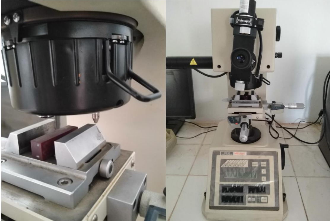
Figure. III.9: Durometer Model MVK-H2 (Hardness Testing Machine).
