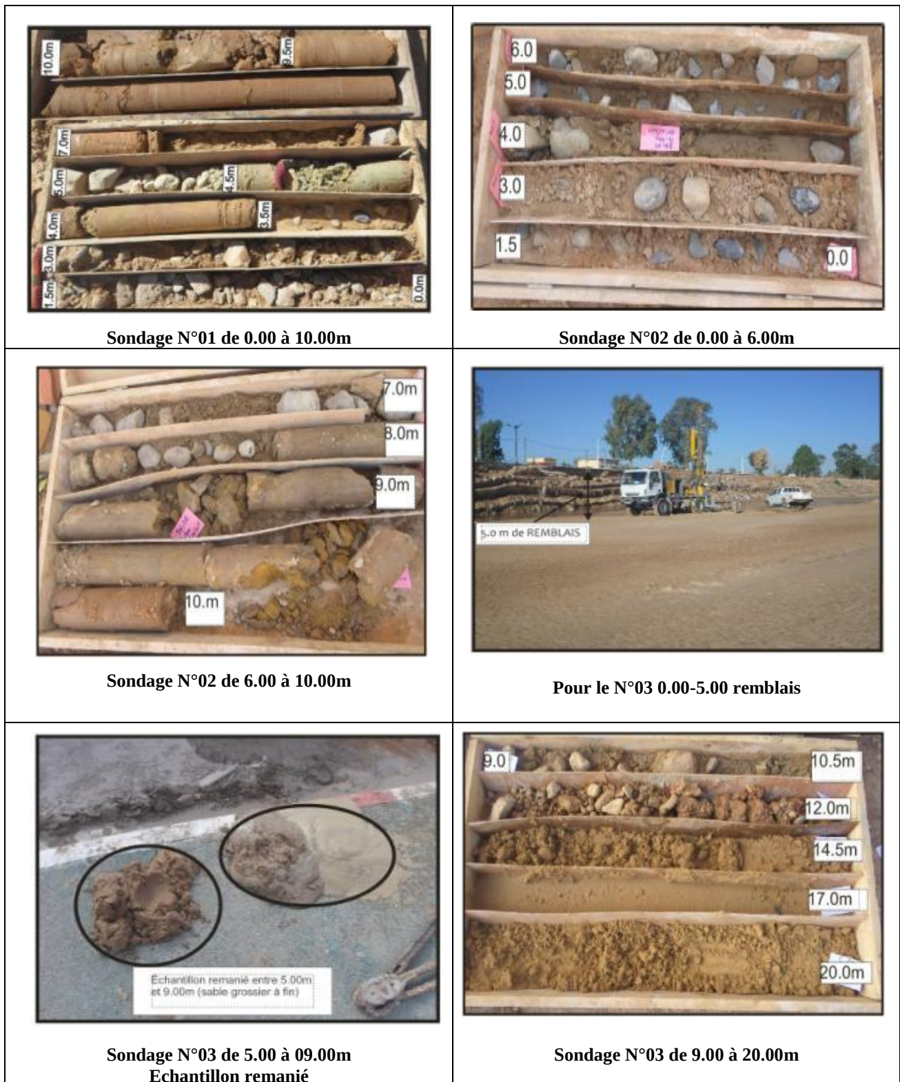
Figure III.2: Photo des caisses de sondage
