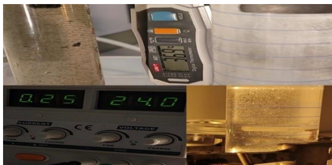
Figure.II.9. The measurements of the produced gases during the water-splitting process
