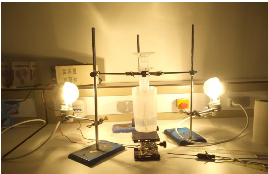
Figure.II.8. Experimental set-up for electrolysis test
