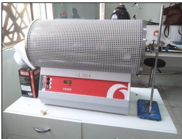
Figure.II.6. Tubular furnace used in the bio-char activation process
