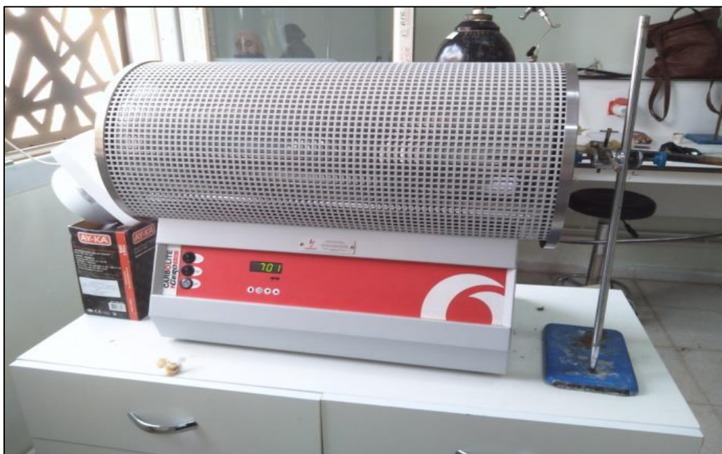
Figure II.6. Tubular furnace used in the bio char activation process
