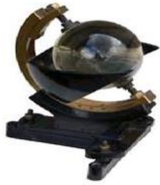
Figure (A-02) : héliographe De Campbell-Stokes.
