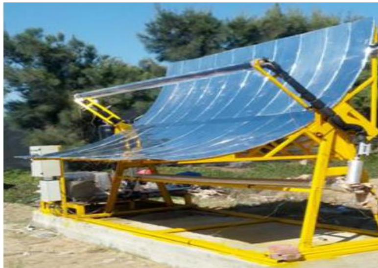
Figure I. 21. The photograph of the experimental device PTC [48].
