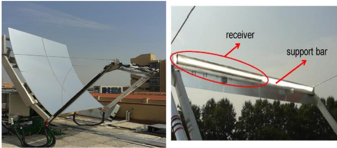
Figure I. 26. (a) Prototype of the asymmetrical parabolic trough linear solar concentrator (b) Bar-and-plate flat receiver arranged on the support bar and illuminated with concentrated solar radiation during a test run [54]
