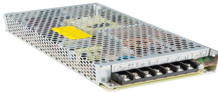
Figure I-1: Real photo of a switching power supplies
