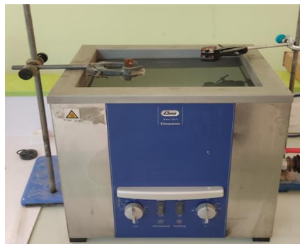
Figure III-5 Bain ultrason Elmasonic Xtra 150H Elma
