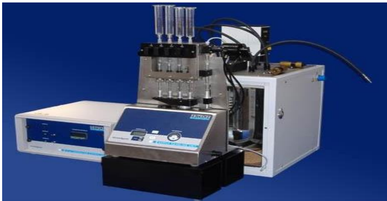
Figure II. 2: Experimental equipment for measuring the CO 2 absorption rate: stopped-flow apparatus
