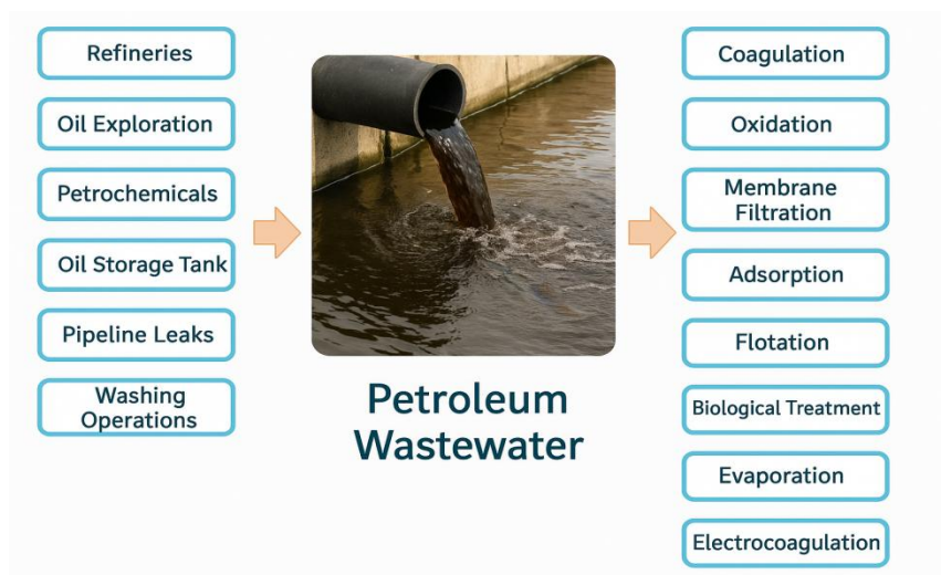
Figure I.1. Conventional and AOPs methods of produced WW.
