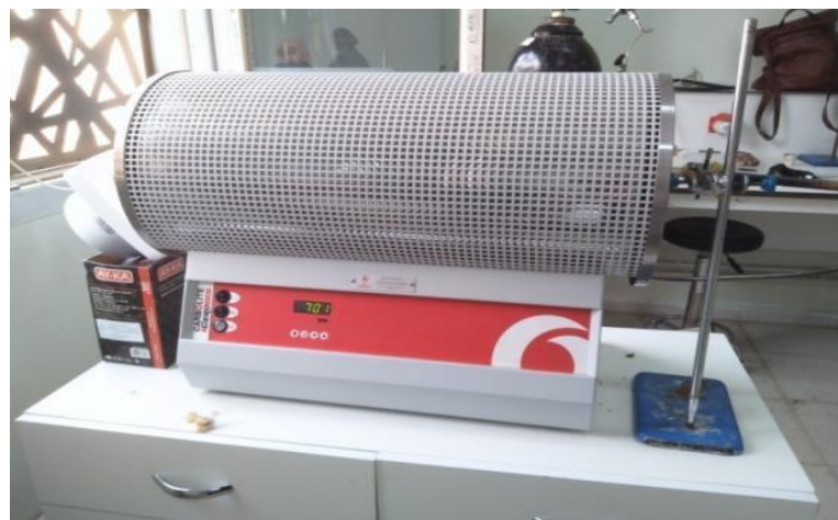
Figure.II.2. Tubular furnace used in the reactivation process of CAC.
