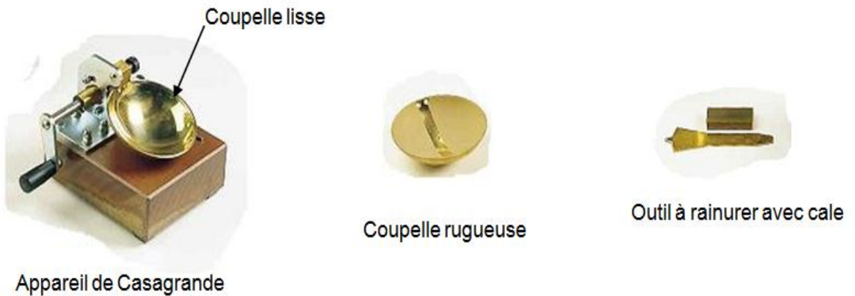
Figure II.4 : Appareil de Casagrande [5]
