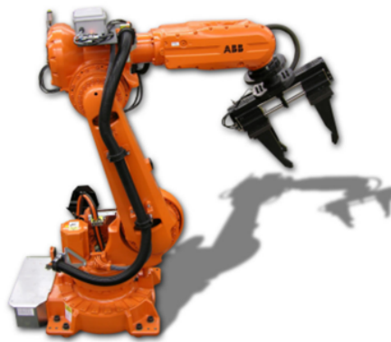
Figure 1.1: IRB6600 from ABB equipped with a spot welding gun
