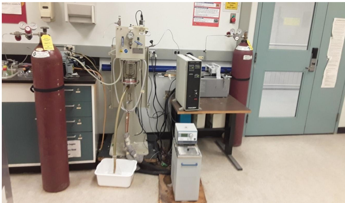
Figure V.1. Solubility experimental equipment for measuring equilibrium solubility of CO 2 (Autoclave reactor).
