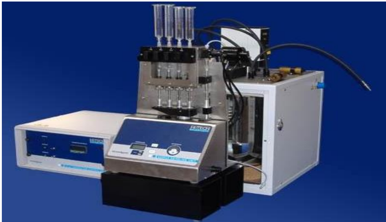
Figure II.2. Experimental equipment for measuring the CO 2 absorption rate: stopped-flow apparatus.
