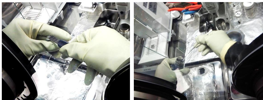
Figure.2: Preparation and weighting of potassium (left) and silicon (right).
