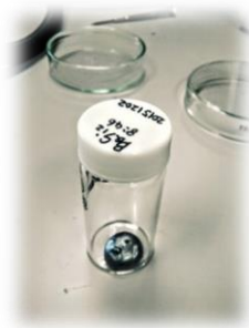
Figure.1: Arc-melted Ba:Si with molar mixture of 8:46
