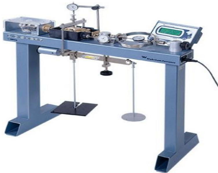
Figure 3-15 Machines de cisaillement direct
