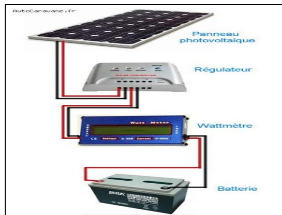
Figure 96: installation Dun Panneaux photovoltaïque
