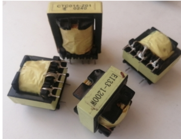
Figure 1.15: Example of transformer Ferrite-based.
