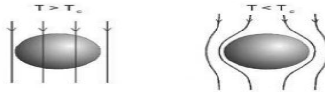
Fig.1. 2. A comparison between how a superconductor acts when it is above and below the T_c [3].
