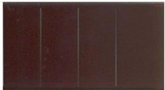
Figure III.12 : Cellule photovoltaïque amorphe [12]
