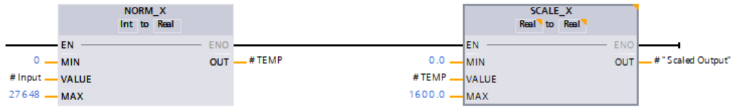
Figure 3.13: Standard scaling function block
