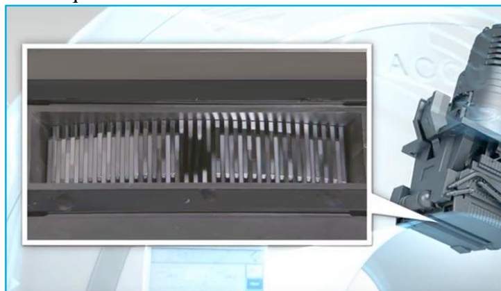
Figure III-2 Real image of Tomotherapy multileaf collimator (MLC).
