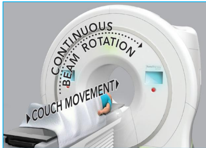
Figure III-10 The gantry rotates around the patient in TomoHelical delivery mode, delivering radiation in a continuous spiral pattern
