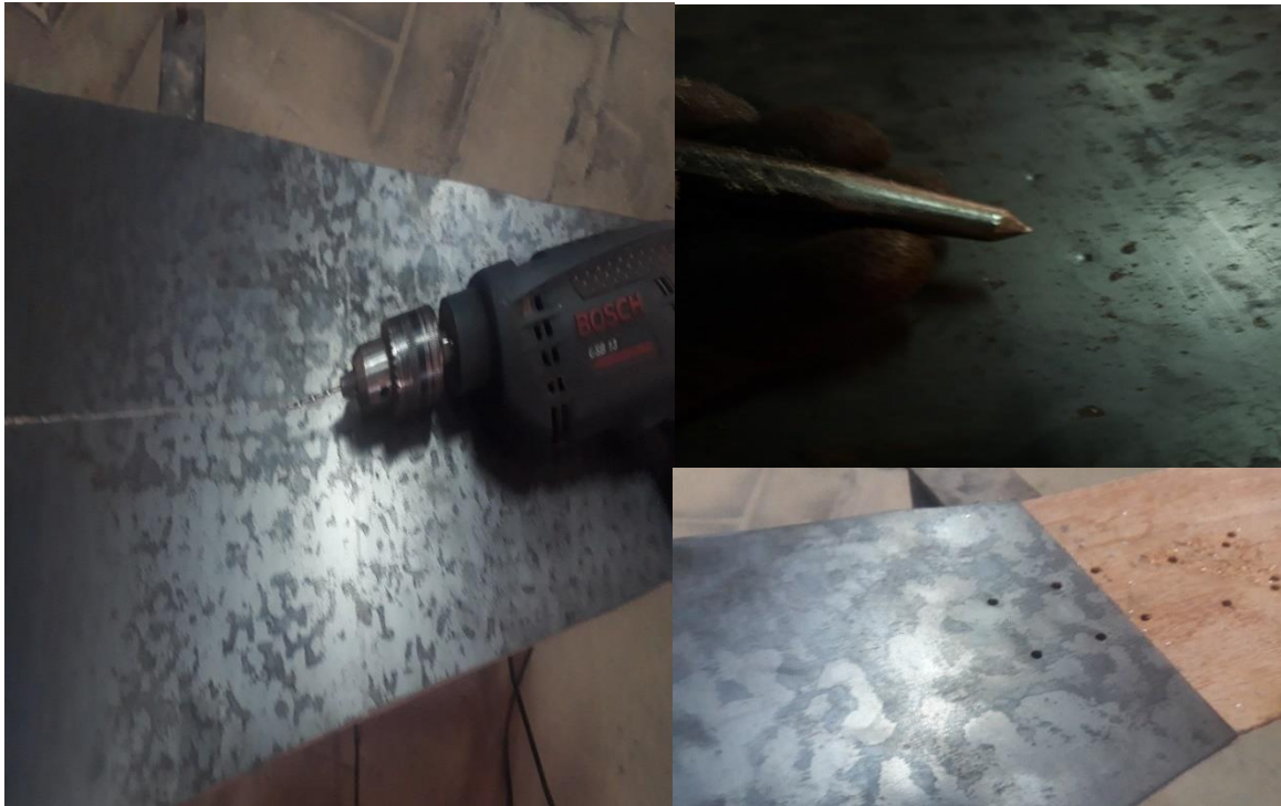
Figure 30: Blade Drilling Process
