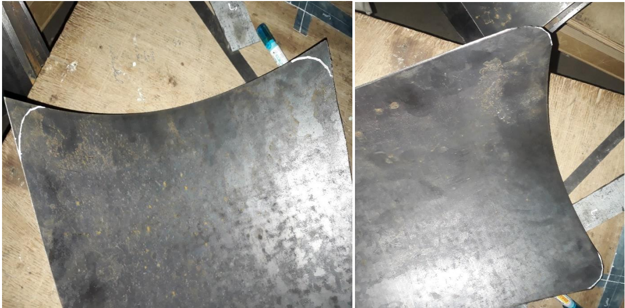
Figure 32: Blade After Cutting
