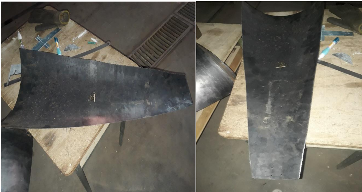
Figure 31: Blade Rolling Process
