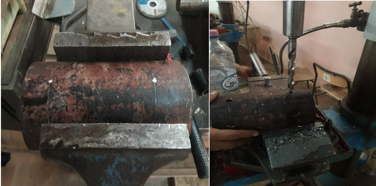
Figure 40: HUB Drilling Process
