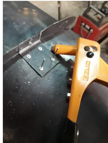
Figure 52: Connect Metal Rip on Blade
