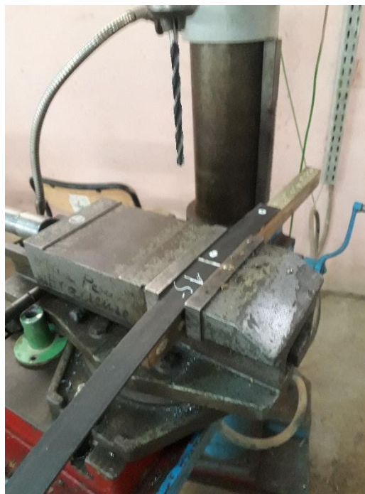
Figure 46: EXT Diameter Drilling Process
