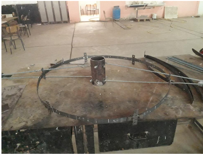
Figure 55: Connect the Hub
