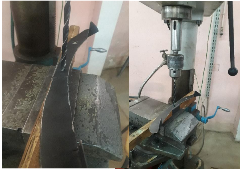
Figure 36: Metal Rip Drilling Process
