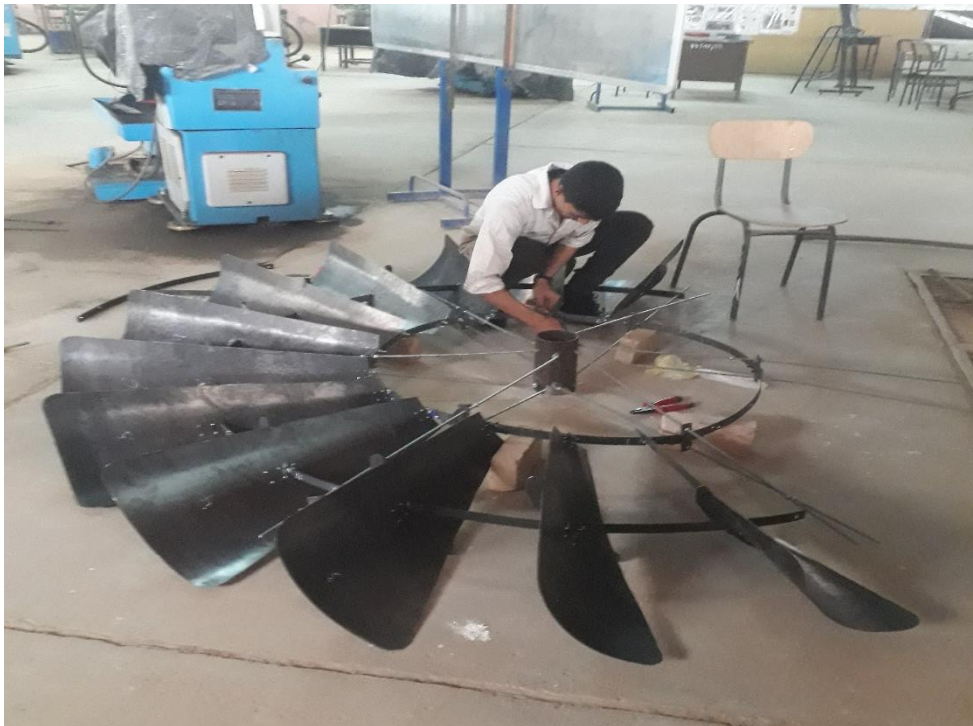
Figure 58: Mounting Blades on HUB Assembly
