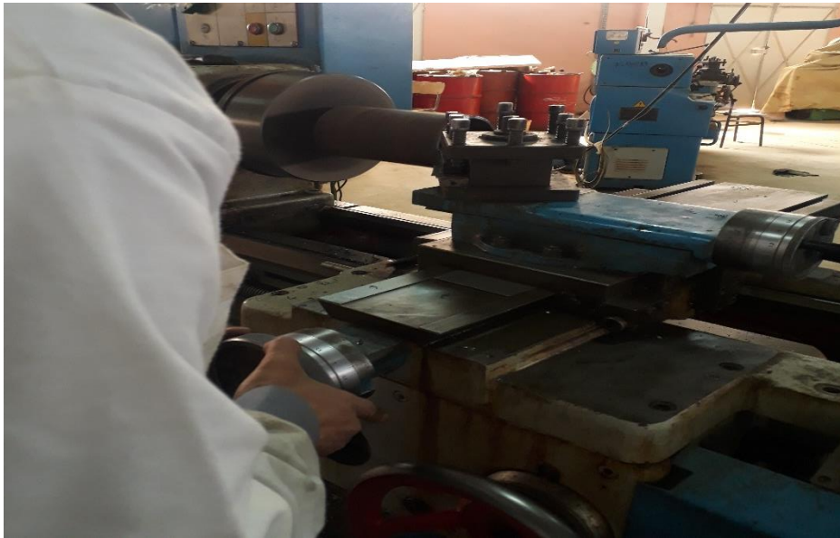
Figure 39: HUB Turning Process
