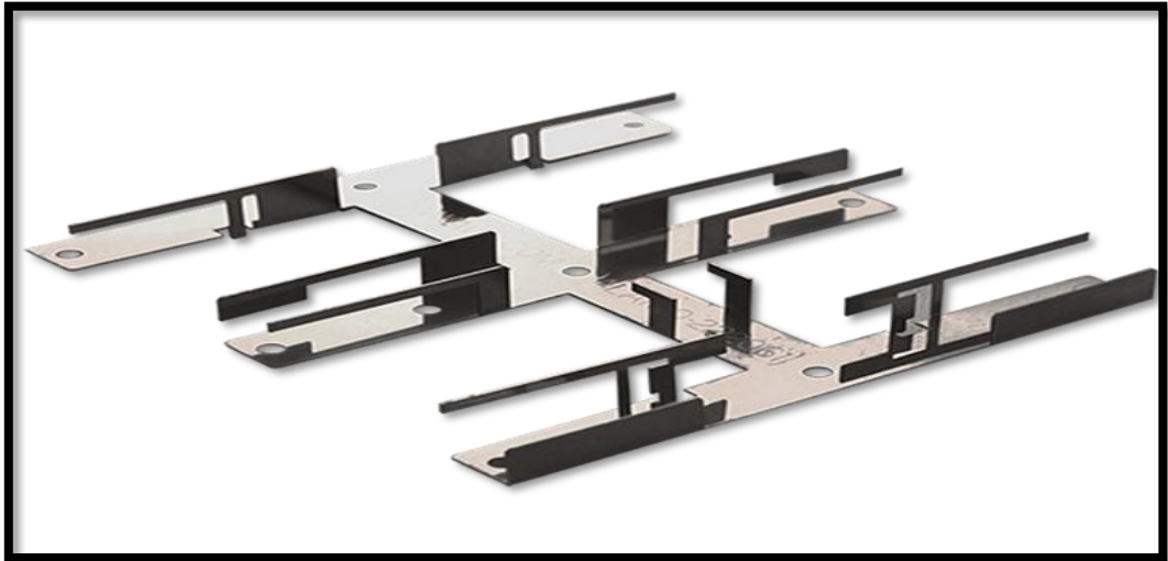
Figure I.5. antenne PIFA multi bande [7].
