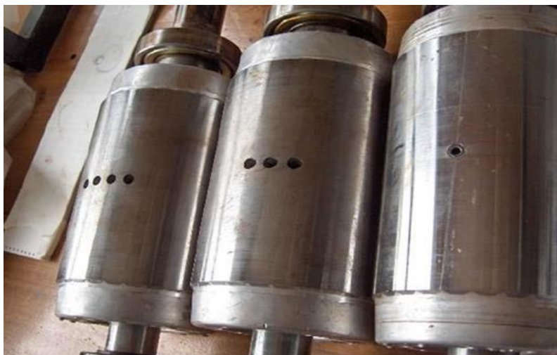
Figure I.11 : Rupture de barre
