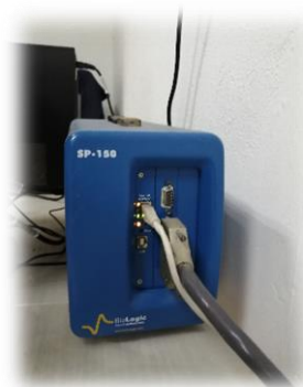
Figure II-8. Potentiostat VoltaLab PGP 201 (a), Potentiostat BioLogic SP150(b)
