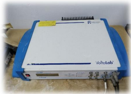
Figure II-8. Potentiostat VoltaLab PGP 201 (a), Potentiostat BioLogic SP150(b)
