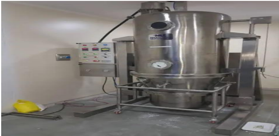
Figure 14: Fluidized bed dryers [41]
