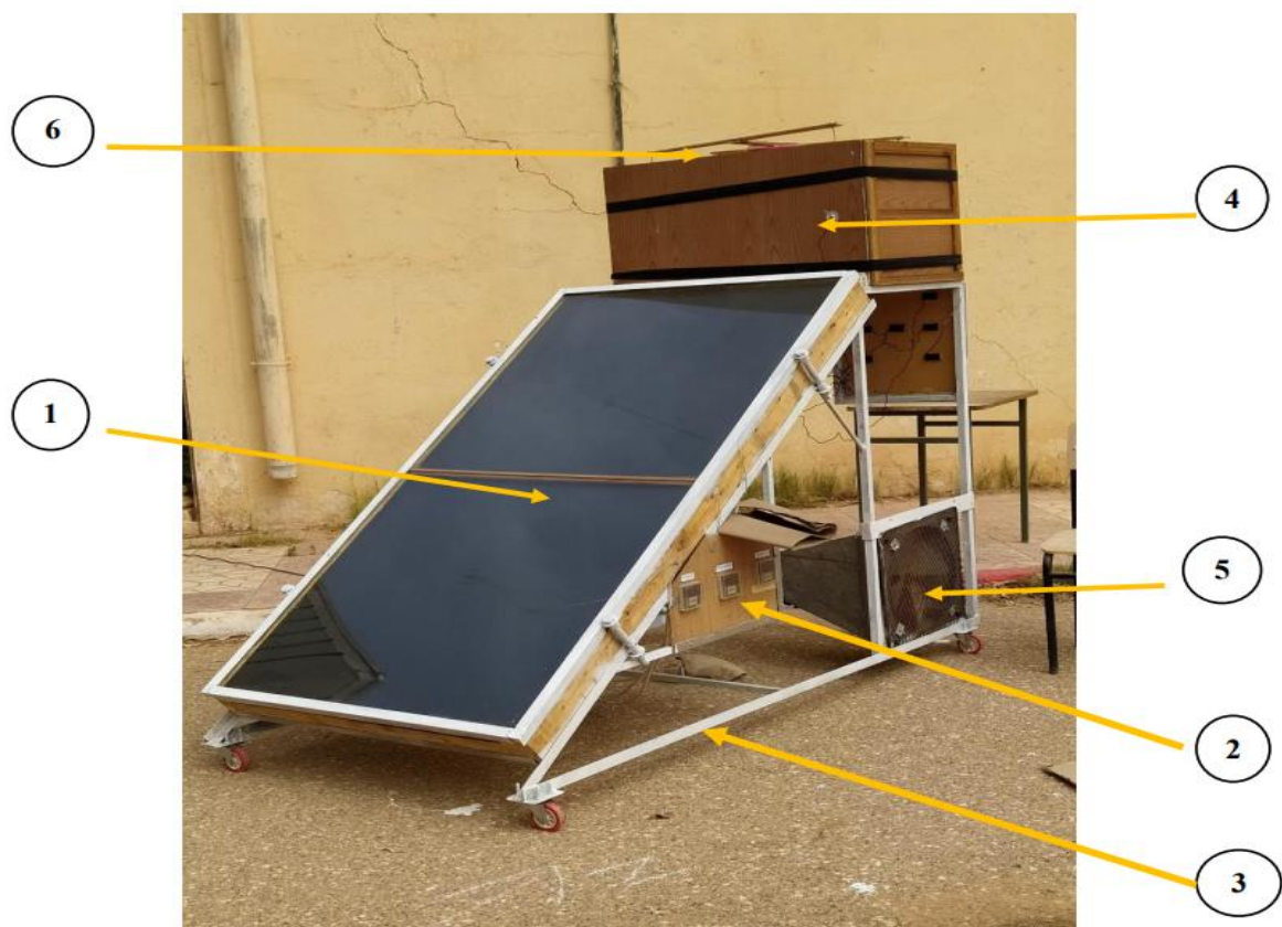
Figure 15: Front view of the test bench.
