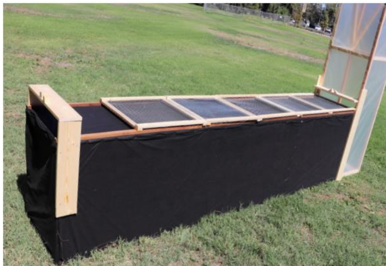
Figure 8: A chimney solar dryer ready for drying fruits and vegetables. Leave the first tray space (left side of photo) empty as a “preheat area. [22]
