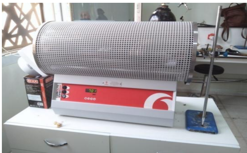
Figure.II.3. Tubular furnace used in the regeneration of EAC
