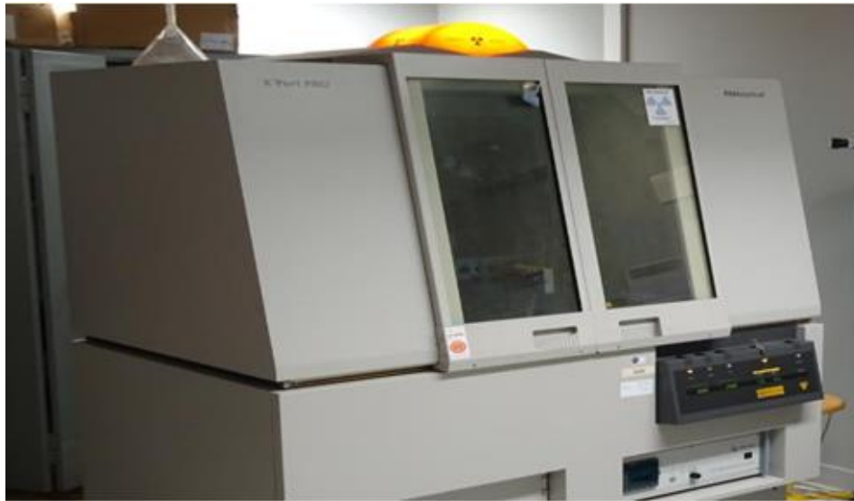
Figure II.2: Diffractomètre PANALYTICAL EMPYREAN
