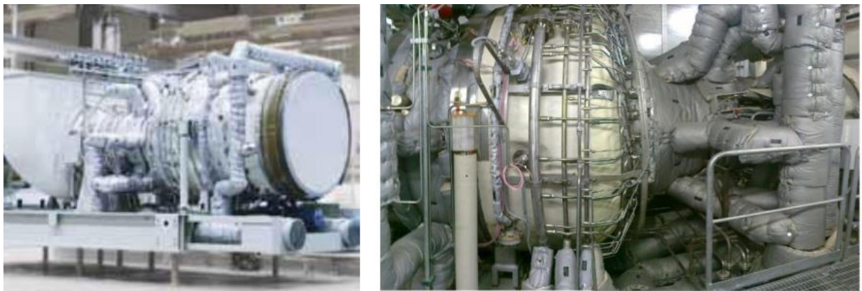
Figure IV 24: SIEMENS SGT-800 gaz turbine power plant
