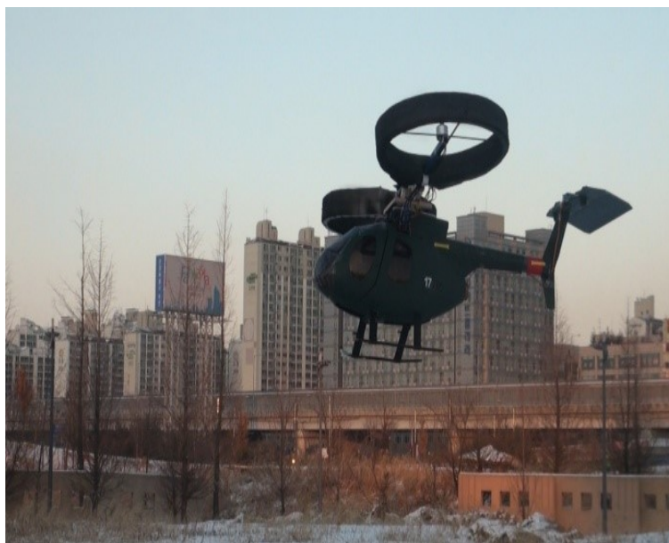
FIGURE 1.14 : Bicopter – 2-Motor Multicopter
