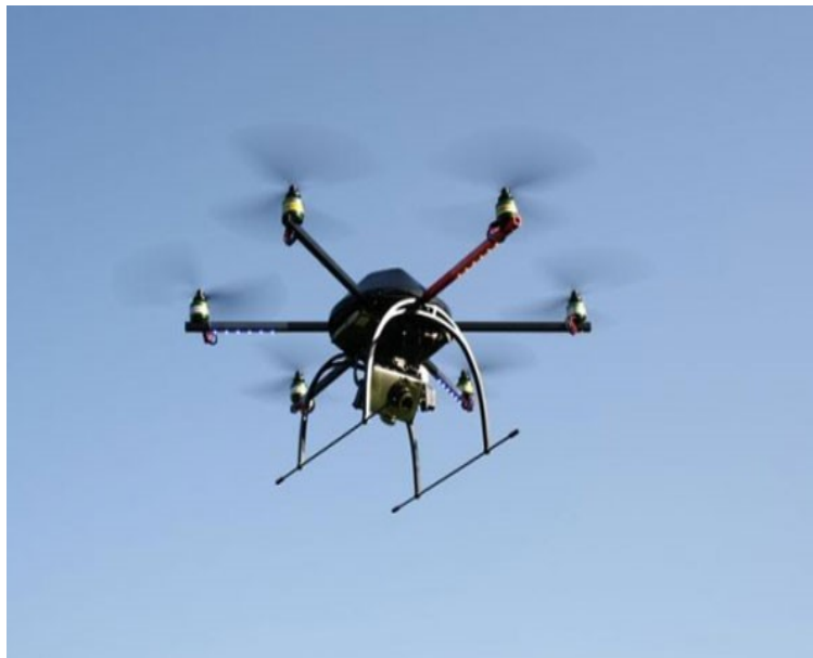
FIGURE 1.17 : Hexacopter – 6-Motor Multirotor
