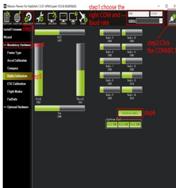
FIGURE 2.23 : Radio Calibration Steps
