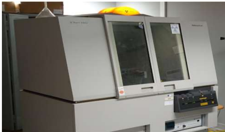
Figure II.3: Diffractomètre PANALYTICAL EMPYREAN
