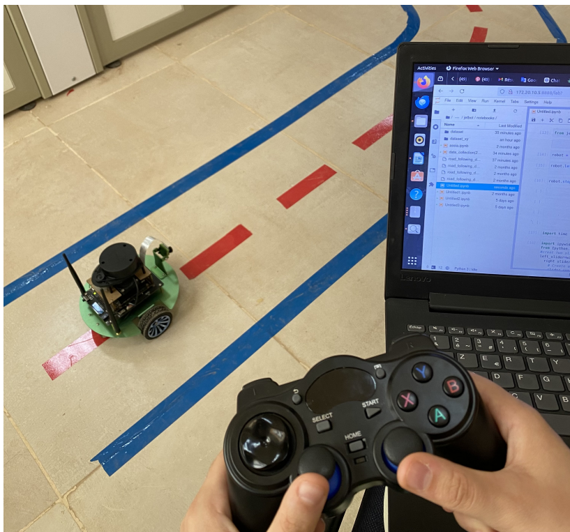
Figure 3.5: driving mobile robot using joy stick.
