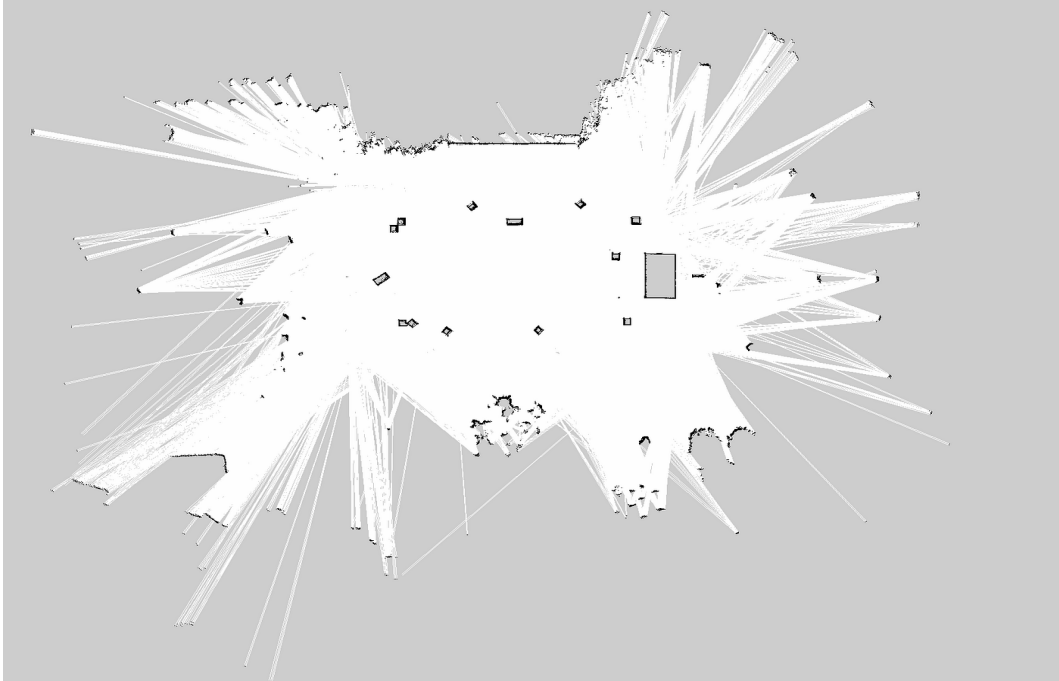
Figure 4.4: Example of a 2-D map created using SLAM based on LiDAR
