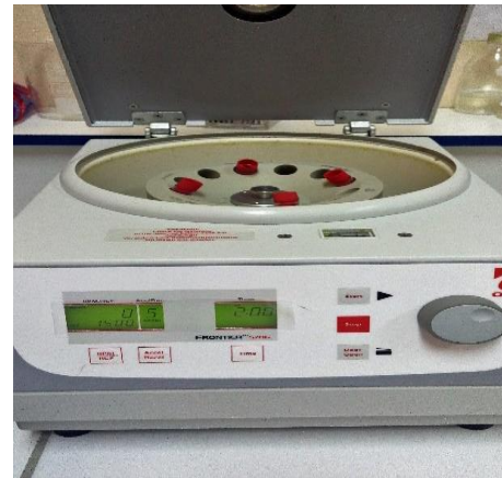
4-Centrifuge 1500 t /m pendant 3min
