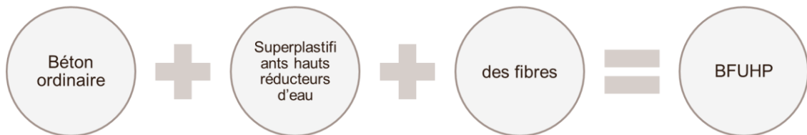
Figure 0-5:composant de beton fibré
