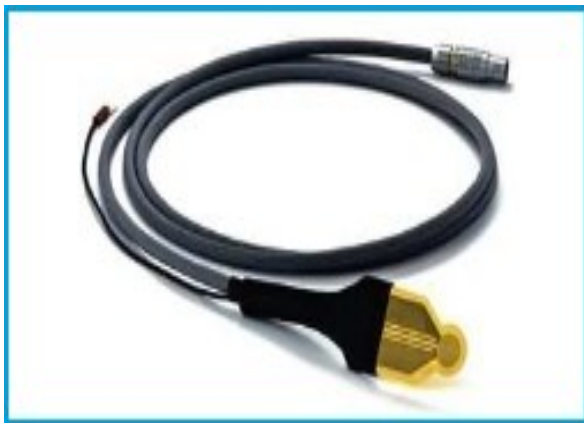
Figure III.26: Photo de La sonde TPS
