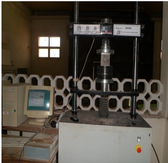
Figure III.22: Essai de compression
