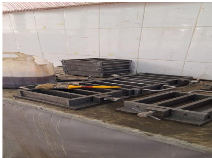
Figure II.37 : Lubrification les moules.
