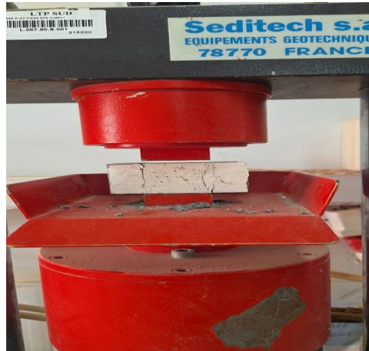
Figure II.42 : Essai de compression.
