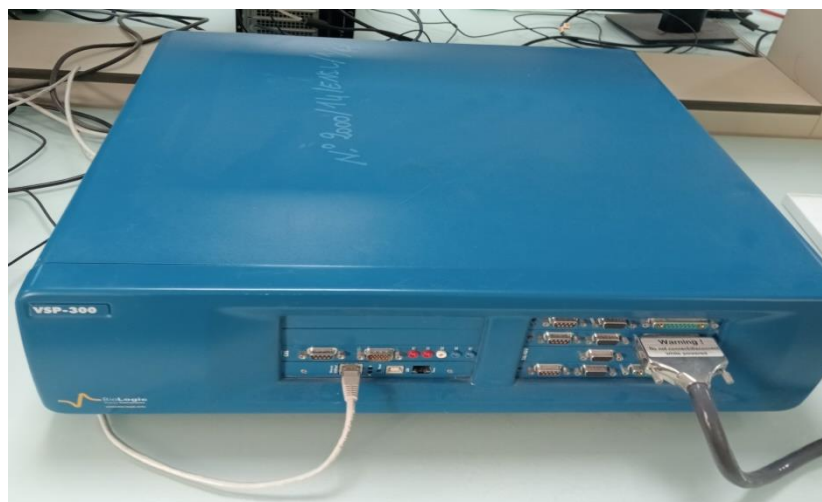
Figure II.2. Potentiostat Biologic (EC-Lab V10.37-VSP-300).
