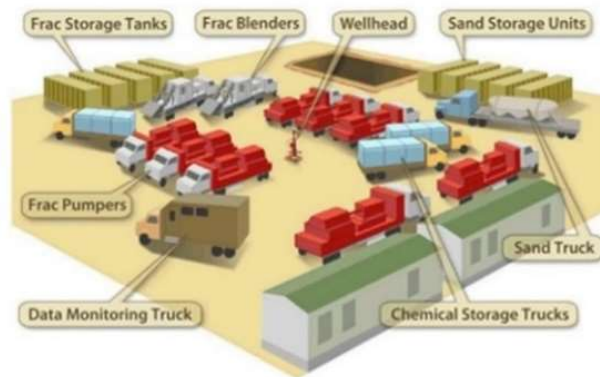
Figure II.1: Hydraulic Fracturing Equipments.
