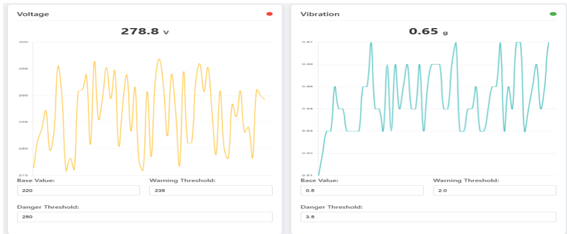
Figure III.14 : Gradual Deterioration (Voltage, Vibration)
