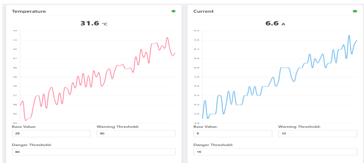
Figure III.13 : Gradual Deterioration (Temperature, Current)
