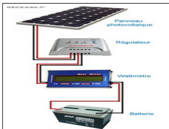
Figure 96: installation Dun Panneaux photovoltaïque
