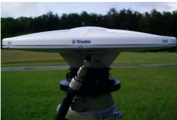
Figure IV.6: Antenne GPS Zephyr Geodetic 2.
