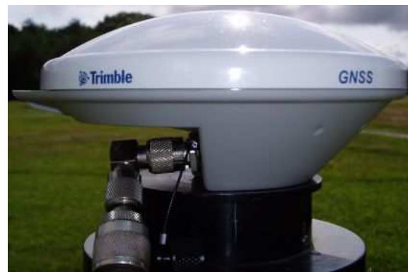
Figure IV.7: Antenne GPS Zephyr - Model 2.
