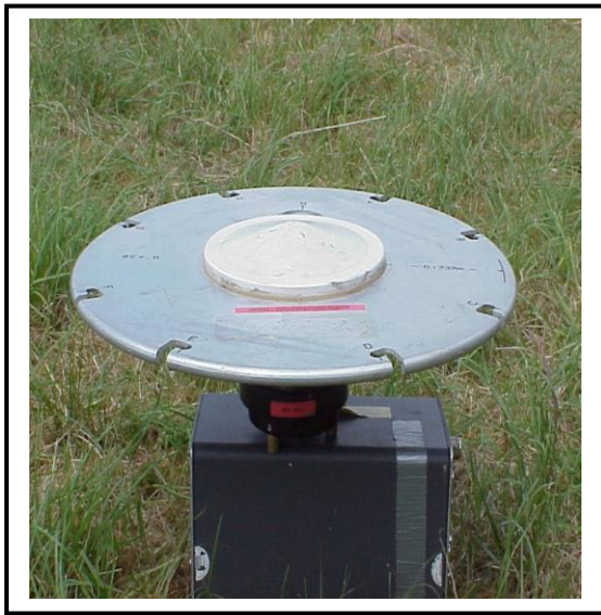
Figure IV.23 : Antenne Ashtech Z-XII3
