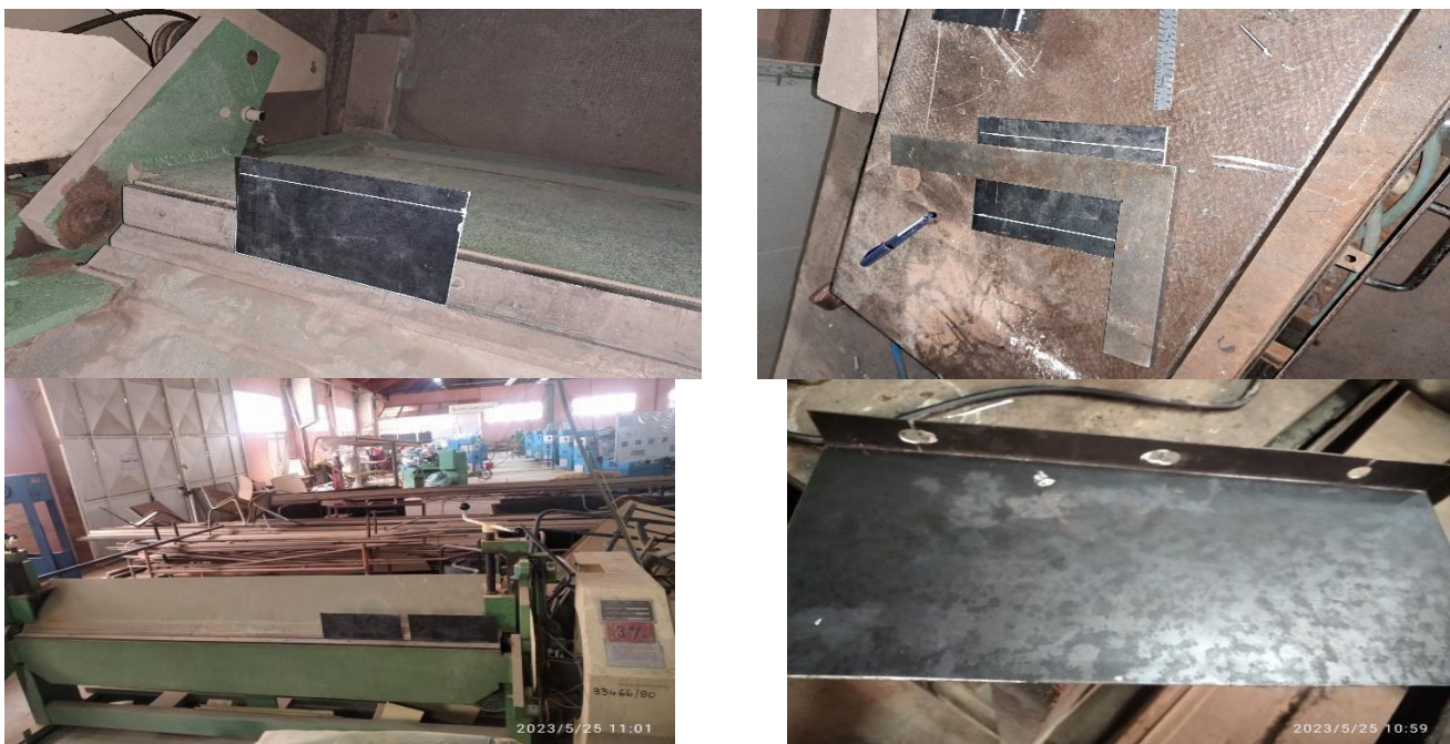
Figure 3.21: Folding, welding and perforation of shaped parts
