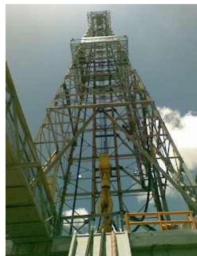
Figure 3. Travelling Block,crown block,drill line and hook
