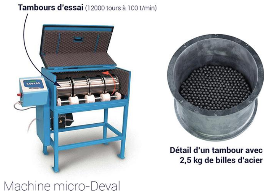
Figure 22. Appareil de Micro-Deval [5].
