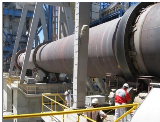
Figure I-6: Four cuisson du gypse [7].
