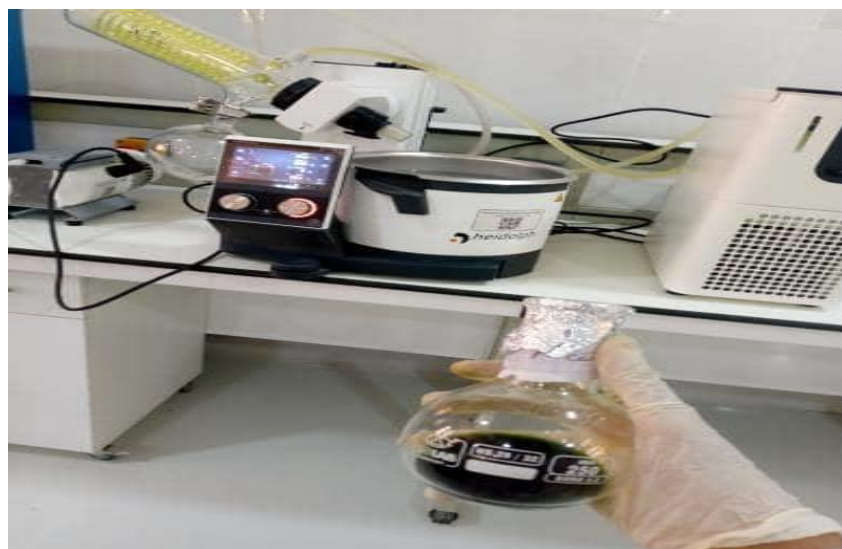
Fig.2.8: Picture showing the evaporation process using the Rotavapor.
